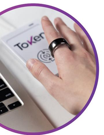
**LED** The multi-color LED indicates status to the user. The light relays a variety of information, including the current battery level, authentication success or failure, BLE/NFC status, and more.
